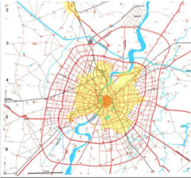
Figure 6: The arterial road grid in the 2011 development plan for Ahmedabad, India, allows for orderly urban expansion.
