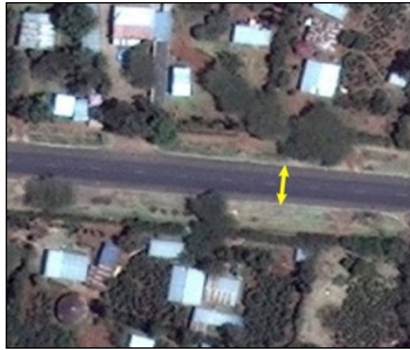
Figure A2: The measurement of the width of a road using Bing satellite imagery as a tracing background.
