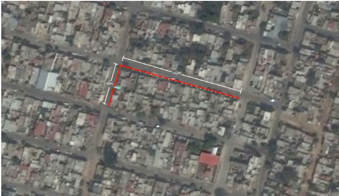
Figure 12: Arriving at a typical plot size in an informal subdivision in Guadalajara, Mexico, by measuring overall block length and depth and dividing each dimension by the number of plots along it.
